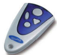
Handsender Mini-Novotron 504 4-Kanal, 433 MHz, KeeLoq-Wechselcode
